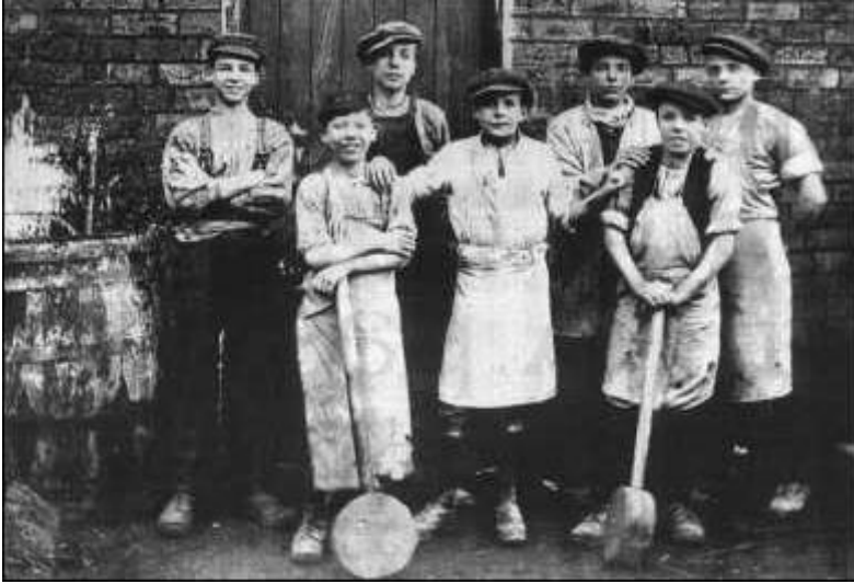
Pottery lads in 1921 with two mawls, the tool used for bottom knocking. Photo: Gladstone Pottery Museum
